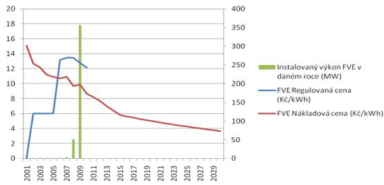
Fig. 1. Regulated price development compared to calculated costs of installation of PV in the Czech Republic. Data up to 2010 are observable, data from 2011 then on are estimates of the author. Left axis shows CZK, right axis shows MWs.
